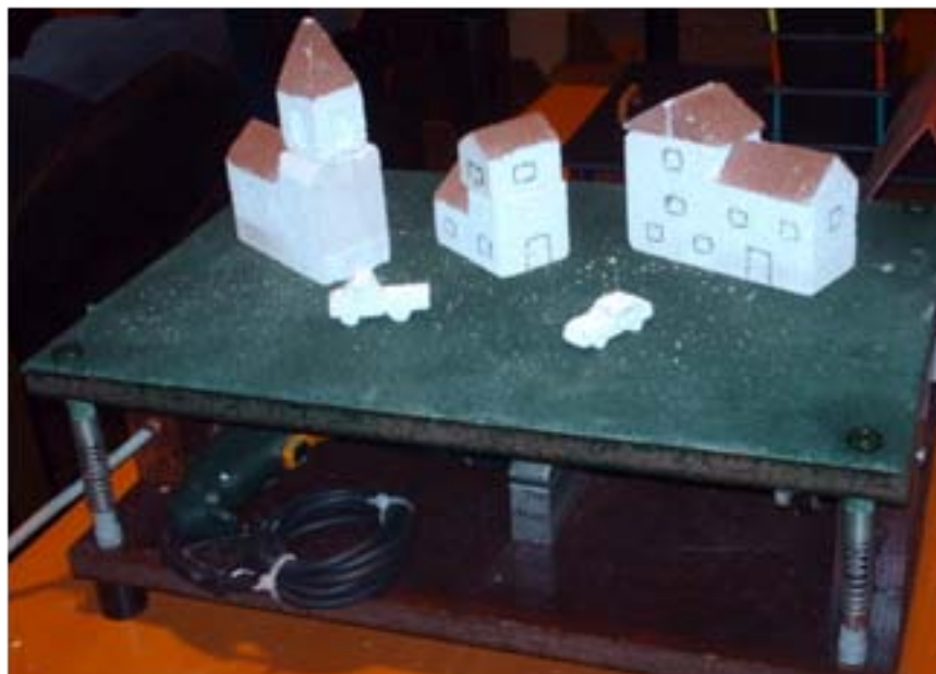
FIG 4. 3_THE VIBRATING PLATE FOR REPRODUCTION OF THE EFFECTS OF AN EARTHQUAKE
